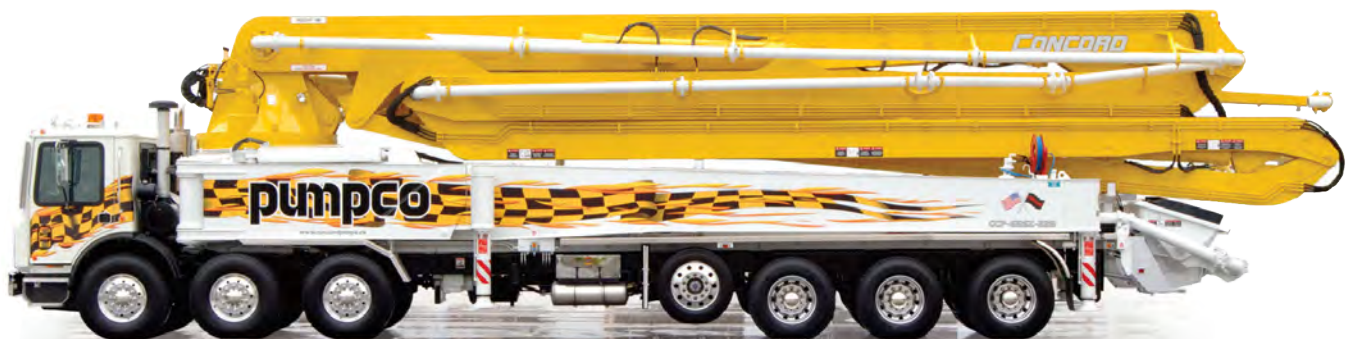
World's first 65-meter boom pump
